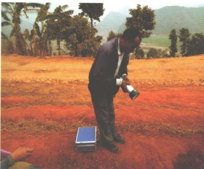
Figure 5: Performing speedy moisture Test at Pipaltar
