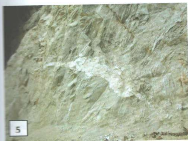
Photo 1) Weathered gneiss, upper part of Salle, L-3. 2) Weathered gneiss, upper part of Salle, L-3. 3) Weathered augen gneiss, road cut section, Kuchipakhel, L-13. 4) Weathered augen gneiss, road cut section, Salle, L-14. 5) Weathered gneiss cross cut with pegmatite vein, Salle, L-15. 6) Metasandstone of Kulekhani Formation, Dharmasthali, L-21.
