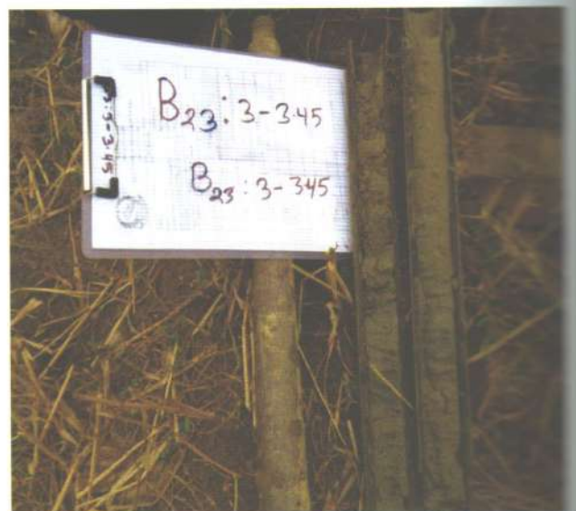
Figure 4: Soil sample from SPT tube
