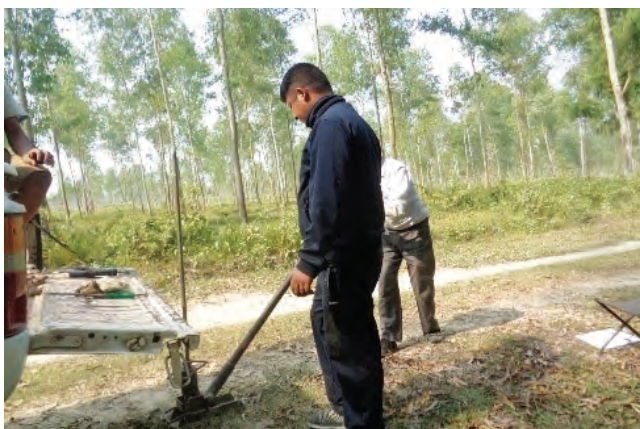
Photo 5. Pulling out the rods after power auger
