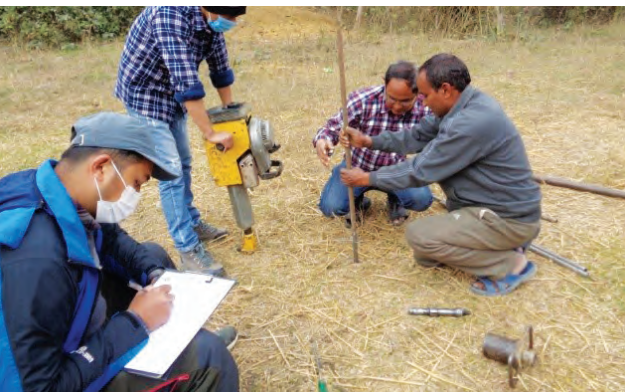
Photo 4: Power auger drilling at site
