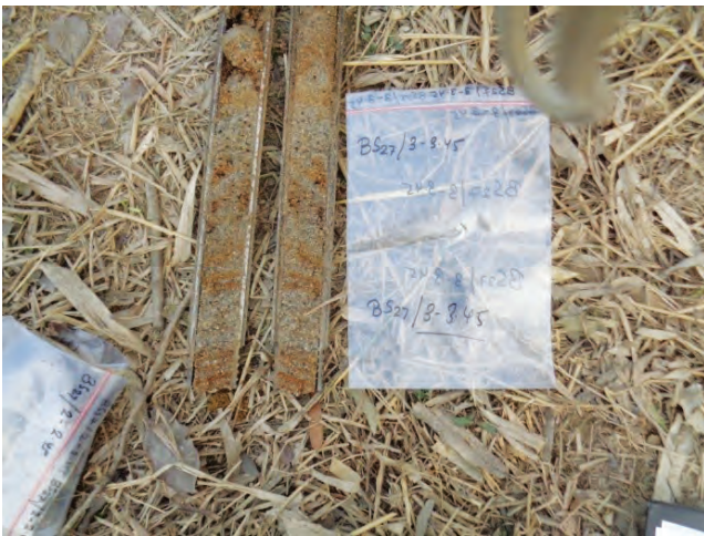
Photo 3: Sample recovered from SPT test
