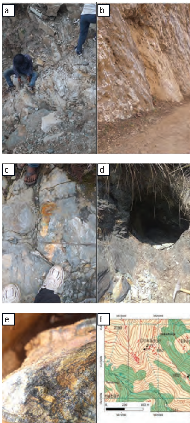
Fig. 3: Gold host rock occurrences a) Cp, py bearing sericitic white quartzite, chloritic quartzite(RC-23,10) b) Shear zone, altered thin bedded marble and pelites (RC 21) c) Chloritic schist with quartz veins(RC11) d) Cu old audit, magnetite, cp, py bearing chloritic schist(RC5), e) Psammitic schist magnetite veins(RC22), f) Location of Au bearing samples
