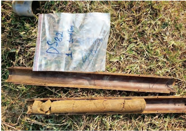
Photo 3. Sample recovered from SPT test
